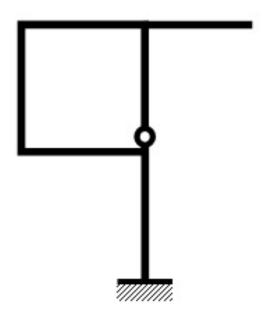
Statically Indeterminate to the second degree
