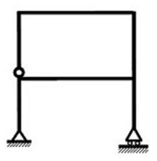
Statically Indeterminate to the second degree
