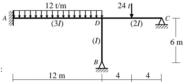
For the shown frame, use the **moment distribution method** to draw the bending moment diagram.  $EI$  is constant.
