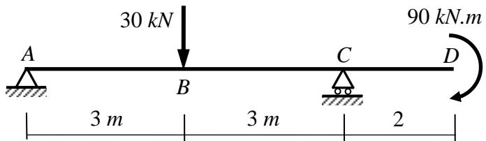
1. The vertical reaction at the roller support **C** is:
