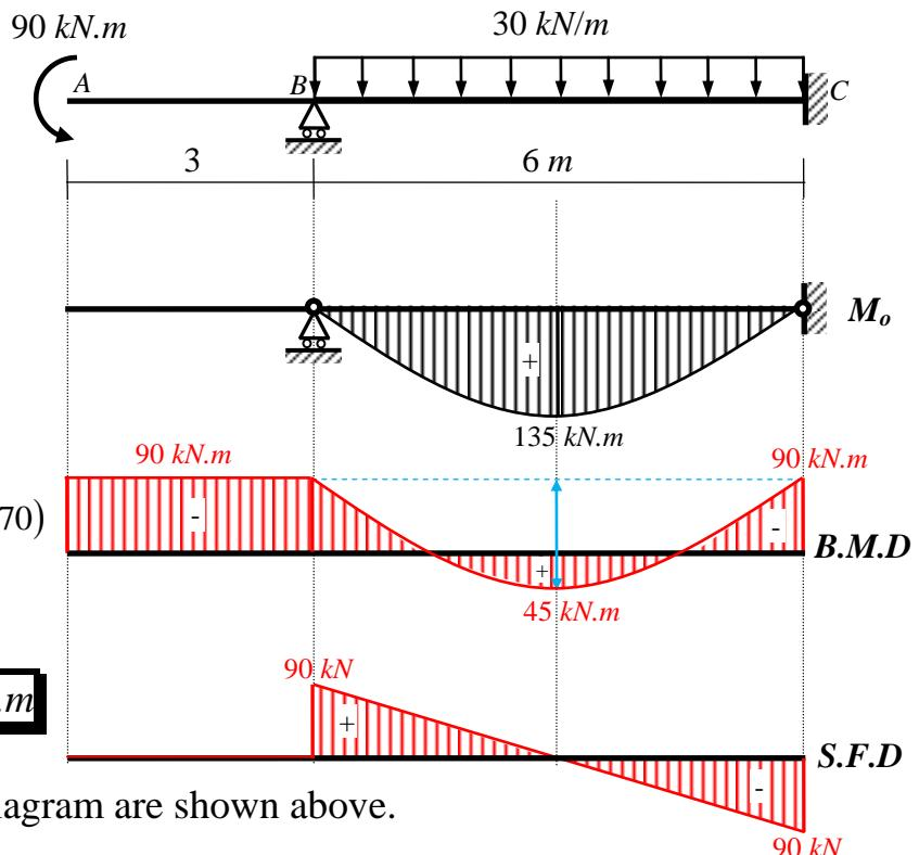
The bending moment and shear force diagram are shown above.
