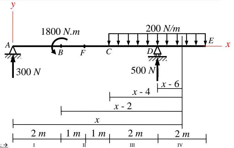
$$\begin{aligned} M &= 300x \left| \begin{array}{l} I \\ -1800(x-2)^0 \end{array} \right| - 200(x-4)^2/2 \left| \begin{array}{l} II \\ III \end{array} \right| + 500(x-6) \left| \begin{array}{l} IV \end{array} \right| \\ &= 300x \left| \begin{array}{l} I \\ -1800(x-2)^0 \end{array} \right| - 100(x-4)^2 \left| \begin{array}{l} II \\ III \end{array} \right| + 500(x-6) \left| \begin{array}{l} IV \end{array} \right| \end{aligned}$$
