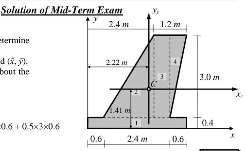
$$S_y = \sum A_i x_i = (3.6 \times 0.4)(1.8) + (0.5 \times 3 \times 1.8)(1.8) + (3 \times 0.6)(2.7) + (0.5 \times 3 \times 0.6)(3.2) = \underbrace{15.192 \, m^3}_{2.5 \times 1.8}$$
