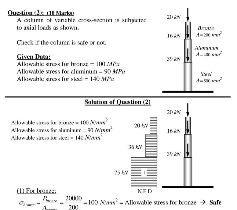
(2) For aluminum:  $\sigma = -\frac{P_{alum}}{2} - \frac{36000}{2} - 90 \ N/mm^2 - Allowable stress for aluminum \rightarrow Safe$
