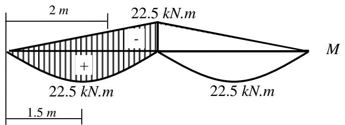
$$\begin{aligned} (a) \theta_A &= \frac{1}{EI} [Area_{AC}] \\ &= \frac{1}{20000} \left[ \frac{2}{3} \times 3 \times 22.5 - \frac{1}{2} \times 3 \times 22.5 \right] = \frac{11.25}{20000} = 5.625 \times 10^{-4} \text{ rads} \\ &= 0.0322 \text{ degrees} \end{aligned} \quad \therefore \boxed{\theta_A = 0.0322^\circ}$$
