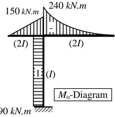
$$\delta_{cv} = \int \frac{M_o M_2}{EI} dL = \frac{1}{EI} [(-4 \times 90)(2)] + \frac{1}{2EI} [(-\frac{1}{2} \times 2 \times 150)(-\frac{2}{3} \times 2)] = \frac{-620}{EI} \therefore \delta_{cv} = -\frac{620}{20000} = 0.031 \text{ m} = 31 \text{ mm} \uparrow$$
