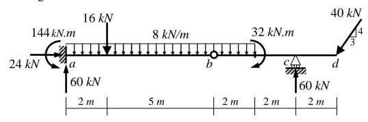
(b) For the shown frame, draw the normal force, shear force and bending moment diagrams. **Note**: The reactions are given.
