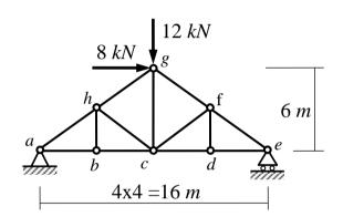
(b) Determine whether each of the shown structures is stable or unstable. If stable, determine whether it is statically determinate or indeterminate. If statically indeterminate, determine the degree of indeterminacy.
