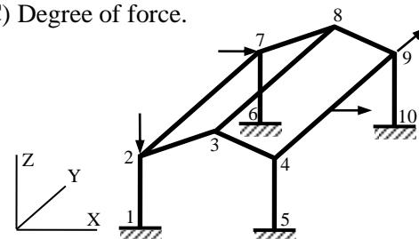
For the shown loaded plane frame with variable moment of inertia, use the stiffness method and neglect axial deformation:
